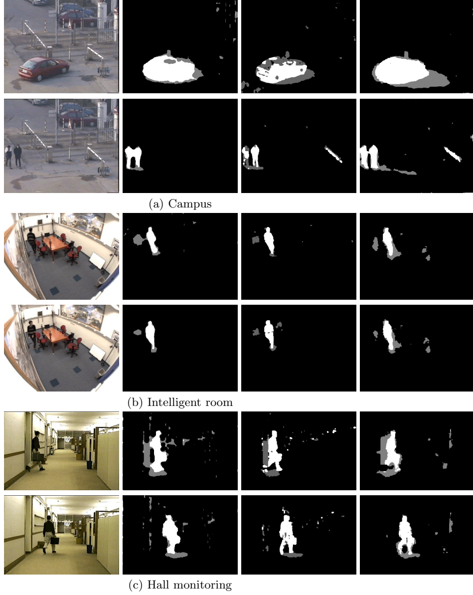
Fig. 6. Some background subtraction results of different methods. The white and gray pixels indicate the detected foreground and shadow regions. First column: original image. Second column: the results by Zivkovic [6]. Third column: the results by Zeng [14]. The right-most column: the results by the proposed method.
